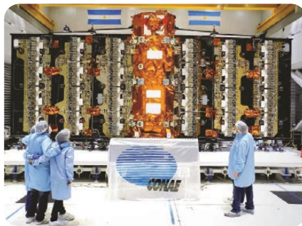
SAOCOM-1A with its radar antenna deployed
